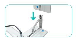
**b.** Slide a lower extrusion onto corner extrusion.
