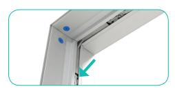
c. Push latches into extrusion groove to lock into place.
