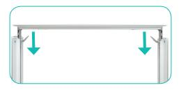
**b.** Attach top extrusion onto frame. **Note:** Before installing top extrusion, remove the top edge-light strip on each side of the frame.
