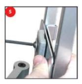
SCREW TOGETHER THE MONITOR BRACKET, INTERFACE MOUNT AND MOUNTING BRACKET TO THE TRUSS LENGTH USEING T-TOOL.
