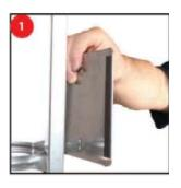
PLACE MOUNT ON TRUSS IN DISIRED LOCATION, USING THE MAGNETS TO HOLD IN PLACE.
