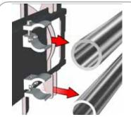
Install monitor mount and TC-30 brackets in the center of tablet kiosk frame.
