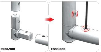
Compress one unlocked end of the connector and slide it through one tube end. Compress the other end of the connector and slide the second tube on. Lock both screws carefully using your allen key tool. Be sure to lock securely, but do not overtighten.
