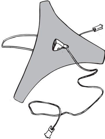
1. Feed power and video cables through the hole in the base.
