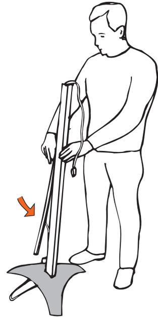
3. Pull off the plastic channel cover and run the cables underneath. Reinstall the cover over the cables.
