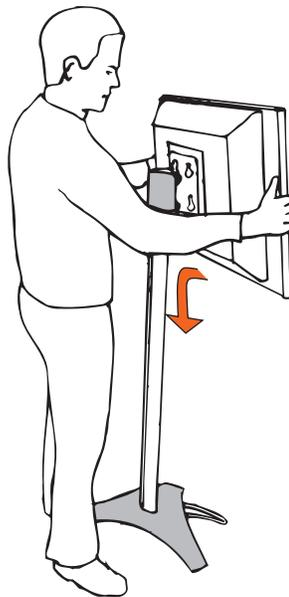
5. With the adapter plate mounted to the back of the monitor, align the four key holes together and slide the monitor down into place.
