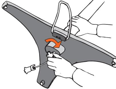
2. Insert vertical pole and tighten the nut on the bottom
