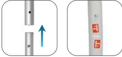
Push down on the button and insert into the receiving tube until the button snaps in place. Match the labels, located on the ends of every piece(ex:T1:T1,T4:T4,etc.).
