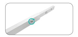
**b.** Tighten screw to lock it into place. Remove the remaining screw from the connector.
