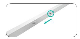
**c.** Then slide the other extrusion onto split connector. Make sure extrusions are flush and tighten the screw to secure connection.
