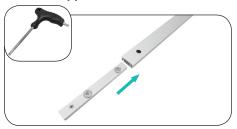
a. Remove screws from Center Connector.
