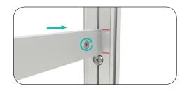
**c.** Add a second support strut to align marked lines and tighten screws with torx key to secure connection.
