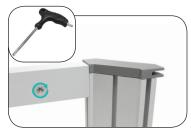
**d.** Connect the top extrusions together and use torx key to tighten.
