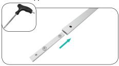
a. Remove screws from Center Connector.
