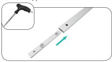
a. Remove screws from Center Connector.
