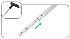
a. Remove screws from Center Connector.
