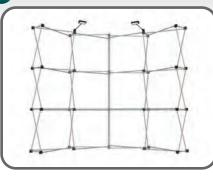
Pull the frame straight up from the center to a full erect position and fasten spacer bars.
