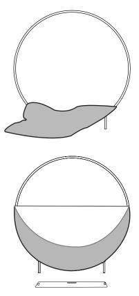
Drape bottom of graphic over the bottom of the frame. Thread the "legs" through and insert them into the base. Pull graphic halfway up the frame.
