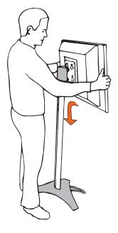
5. With the adapter plate mounted to the back of the monitor, align the four key holes together and slide the monitor down into place.
