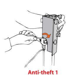
4. For a VESA 200x200 mounting pattern, mount the adapter to the vertical pole and tighten the nuts for theft protection.
