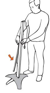
3. Pull off the plastic channel cover and run the cables underneath. Reinstall the cover over the cables.
