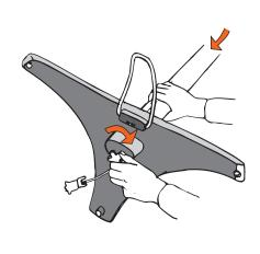
2. Insert vertical pole and tighten the nut on the bottom
